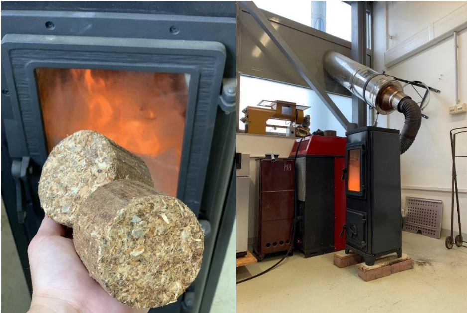
Figure 13 Mango pits briquettes and its combustion test
