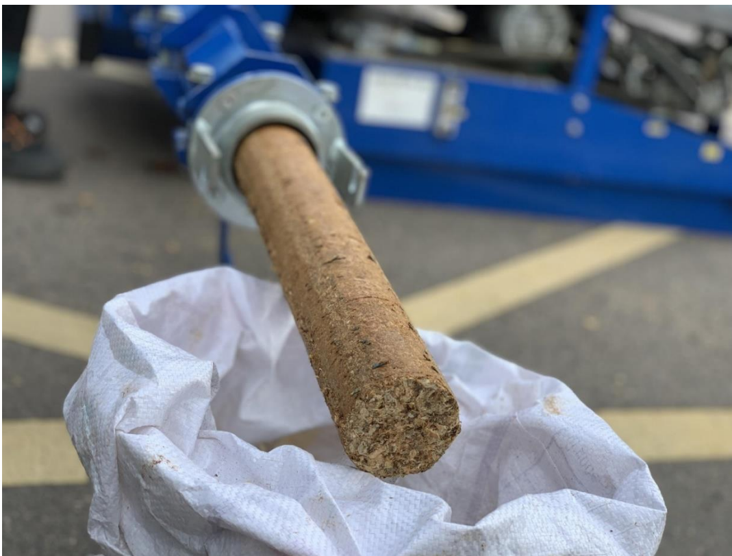
Figure 12 Pilot fabrication of mango pit fuel briquettes
