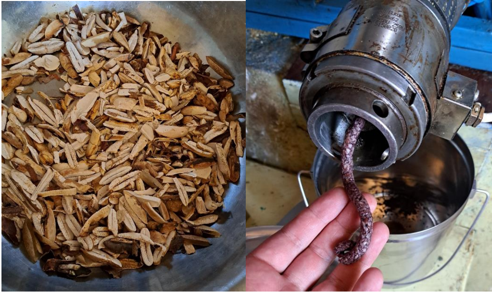
Figure 112 Pieces of cut mango kernel and oil extraction machine Farmet Uno
